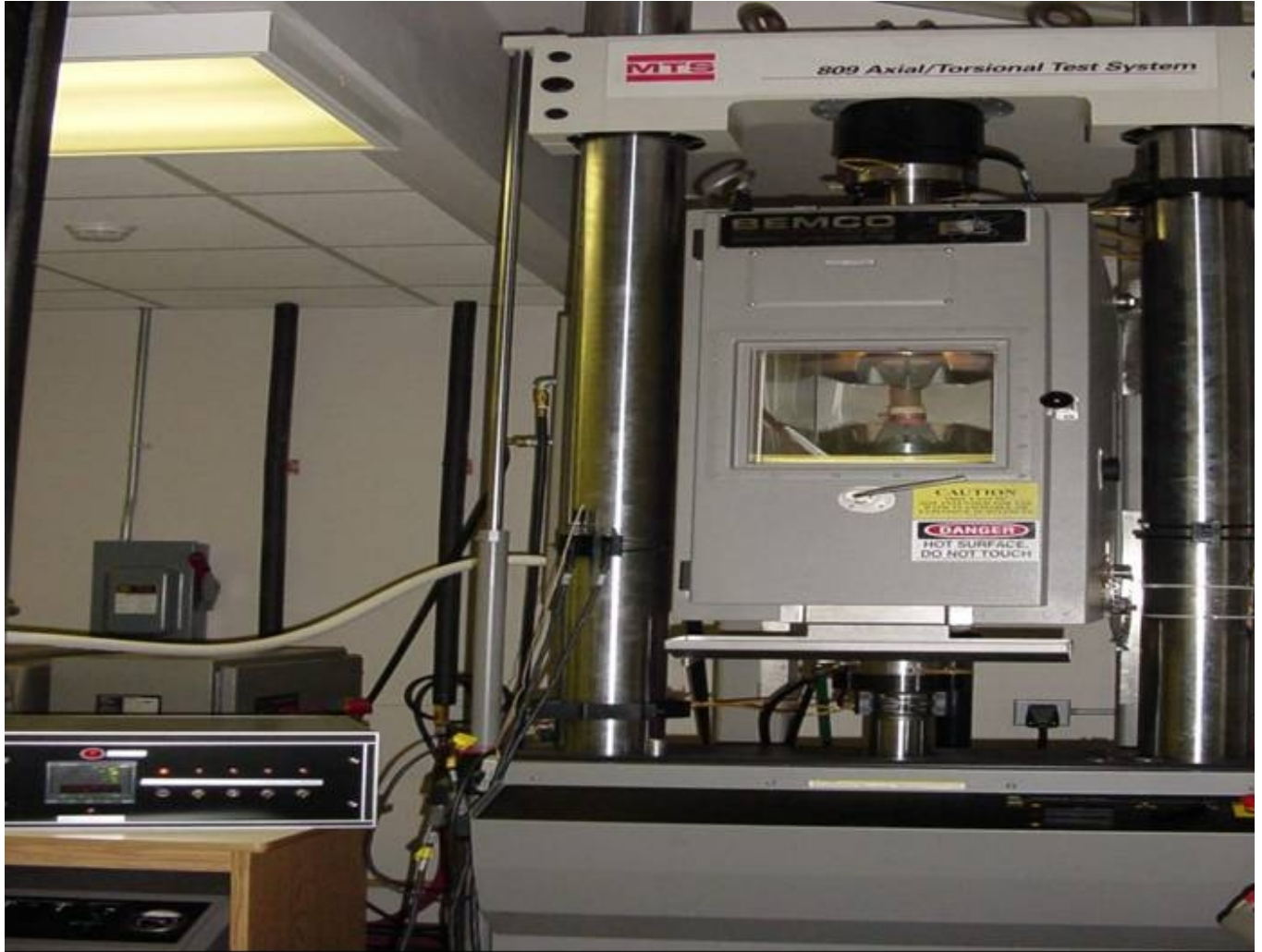
Photo 2: AU-MTS Lab’s 809.10 sophisticated servo hydraulic materials testing system
