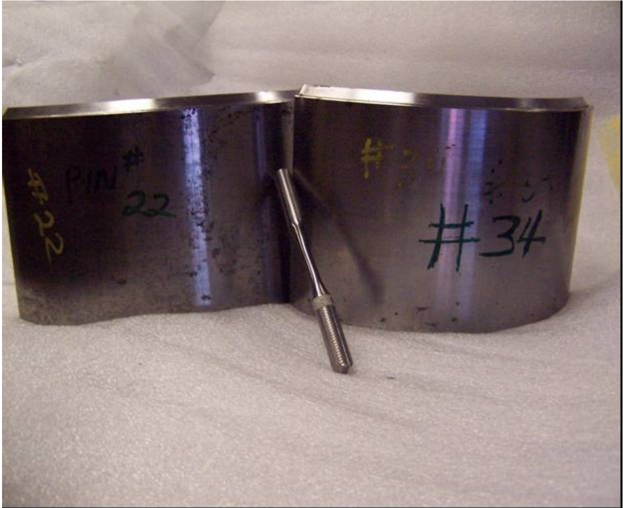
Photo 1: Overlook of XXX Corporation's steel parts of ID #22 and #34 and a fabricated fatigue testing specimen
