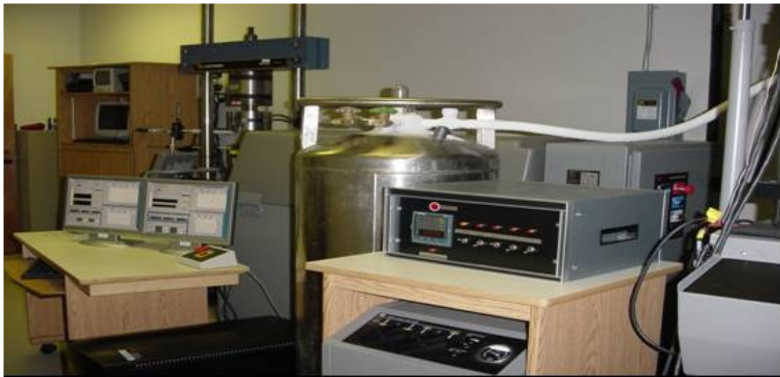
Photo 3: AU-MTS Lab's Instron-1331 sophisticated servo hydraulic materials testing system, its telescope measurement facility, and Nitrogen tank for fatigue testing with temperature below 0 0 C
